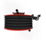
Hose reel designed for fire hydrants. Includes fire hydrant hose and direct/fog nozzle. Equipped with a wall mounting bracket, hose guide, rewinding knob and an automatic valve. Connecting unit size is <sup>3</sup>/<sub>4</sub>. The automatic valve is located in the reel hub. The valve opens when the reel is turned clockwise and closes when the reel is turned counterclockwise. The CE-marked (EN 671-1:2012) fire hydrant reel is always red, and the maximum length of the hose is 30 metres.
