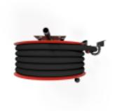
Hose reel designed for fire hydrants. Includes fire hydrant hose and direct/fog nozzle. Equipped with a wall mounting bracket, hose guide, rewinding knob and an automatic valve. Connecting unit size is  $\frac{3}{4}$ . The automatic valve is located in the reel hub. The valve opens when the reel is turned clockwise and closes when the reel is turned counterclockwise. The CE-marked (EN 671-1:2012) fire hydrant reel is always red, and the maximum length of the hose is 30 metres.
