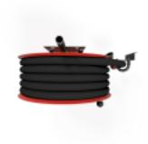
Hose reel designed for fire hydrants. Includes fire hydrant hose and direct/fog nozzle. Equipped with a wall mounting bracket, hose guide, rewinding knob and an automatic valve. Connecting unit size is ¾. The automatic valve is located in the reel hub. The valve opens when the reel is turned clockwise and closes when the reel is turned counterclockwise. The CE-marked (EN 671-1:2012) fire hydrant reel is always red, and the maximum length of the hose is 30 metres.
