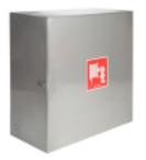
Insulated industrial-grade fire hydrant cabinet with heater, cabinet and reel made of stainless steel. Double insulated door, 19mm cellular rubber heat insulation. Thermostat-controlled electric resistor 200W (230V). Price excludes hose and spray nozzle. Choose hose combination here. Maximum hose sizes 19 mm / 40 m or 25 mm / 30 m, lightweight hose 19 mm / 45 m or 25 mm / 30 m. NOTE! CE-marked EN-671 approved rapid fire hydrant maximum hose length is 30m.
