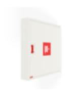
Designed for old buildings where the openings made for old fire hydrant cabinets are used. The cabinet part is 140 mm deep and covers the opening. The cabinet has no back wall, and the reel sinks 100 mm into the old opening. The depth of the cabinet and the size of the reel can be changed if necessary, ask for a quote.
