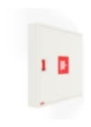
Designed for old buildings where the openings made for old fire hydrant cabinets are used. The cabinet part is 140 mm deep and covers the opening. The cabinet has no back wall, and the reel sinks 100 mm into the old opening. The depth of the cabinet and the size of the reel can be changed if necessary, ask for a quote.
